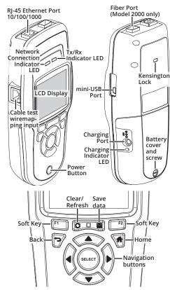
The LinkRunner AT is a portable device that allows networking professionals to easily verify network availability and copper and fiber cable connectivity, identify networks and ports, and generate reports. LinkRunner AT 2000 can act as a packet reflector for performance tests run by other NetAlly testers.
