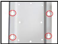
**STEP 5** Stabilize the construct by tightening the four marked screws below figure:
