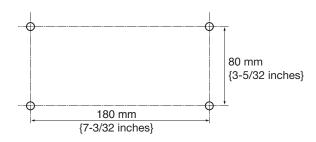
\* The above measurement diagram shows the view when standing on the floor and looking up at the ceiling.
