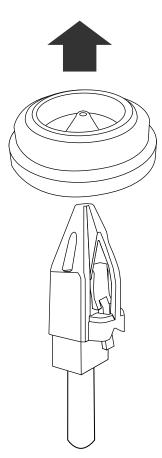
10. Install the silicone seal to its original routing hole.
