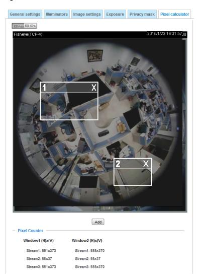
The pixels thus calculated are listed at the lower screen on a per-stream basis depending on the frame size you configured for each video stream. Take the following into consideration when using this feature:
