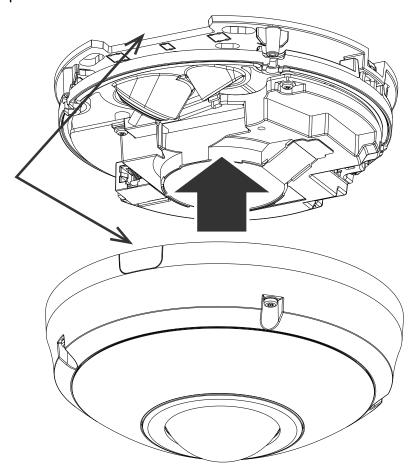
17. Secure the dome cover by fastening the T10 anti-tamper screws.
