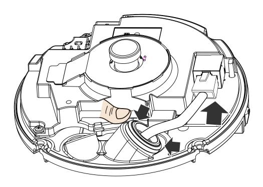
12. Pull the cable slightly backward. Please do not leave the edge of center hole folded toward the inside of the camera. Doing so will compromise its waterproof feature.
