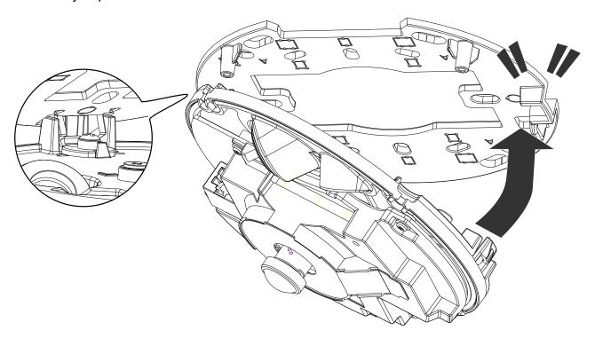
16. Install the dome cover by aligning the side-routing tab with the cabling cut-out on the base plate.
