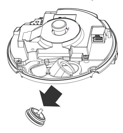
8. Remove the tip of the silicone seal by pulling it off. Insert the RJ45 connector of your Ethernet cable into the penetration cap.
