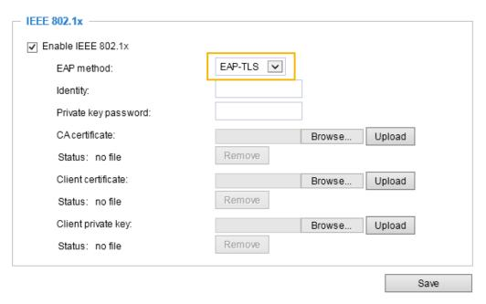
3. When all settings are complete, move the Network Camera to the protected LAN by connecting it to an 802.1x enabled switch. The devices will then start the authentication automatically.
