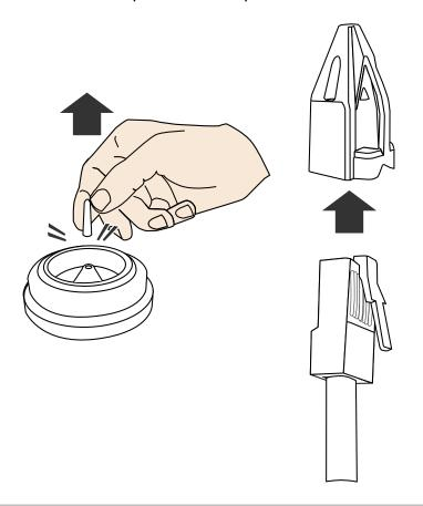
9. Push the penetration cap through the center of the silicone seal.
