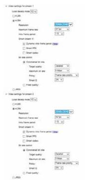
This Network Camera offers real-time H.265, H.264 and MJPEG compression standards (dual Codec) for real-time viewing.
