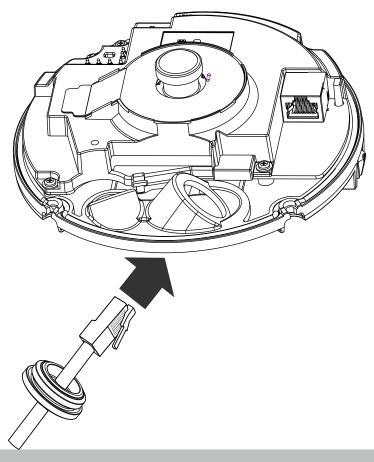
11. Connect the Ethernet connector and secure the top of the silicone seal to the routing hole. You may need to adjust its position.
