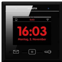
Fig.: After autoconfiguration, the MxDisplay+ is opened in standby mode with date/time display.
