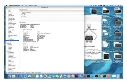
Under "USB 3.0 Bus", you should see an "HDMI to U3 capture". This indicates that your system has successfully discovered CAMLIVE.
