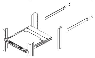
3. After the L-shaped brackets are secured, tighten all the screws.
