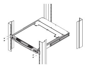
2. While the first person still holds the unit in place, the second person slides the left & right L-shaped brackets into the unit's side mounting brackets from the rear, installing four screws in the brackets to secure them in place.
