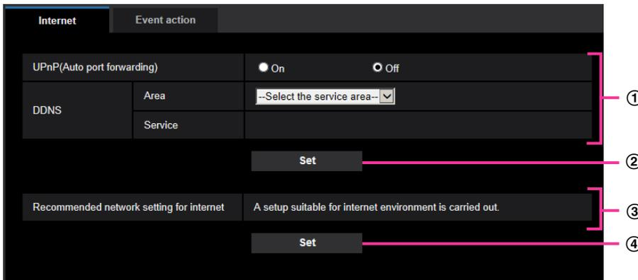
When completing the setting items in field ①, click the [Set] button ② below field ①). The edited settings in field ① will not be applied unless the [Set] button ② below field ①) is clicked. In the same manner as above, click the [Set] button ④) below field ③) when completing the setting items in field ③).
