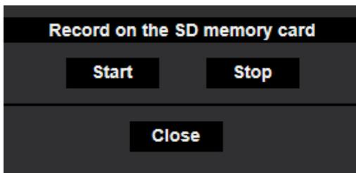
3. Click the [Start] button to start recording images on the SD memory card. The SD recording status indicator will light red (→page 12) while images are being recorded on the SD memory card. The image saving interval can be configured on the [SD memory card] tab of the “Basic” page. (→page 72)
