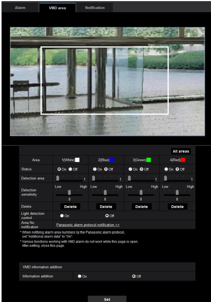
2. Adjust “Detection area” and “Detection sensitivity” using the slider.
