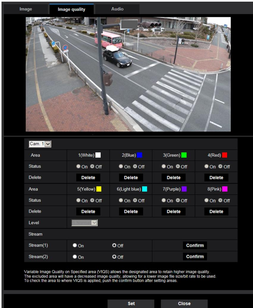
2. Configure the difference level in the image quality between specified areas and non-specified areas. The greater the difference level, the more the image quality of the non-specified area is reduced. This makes it possible to moderate the image data size.
