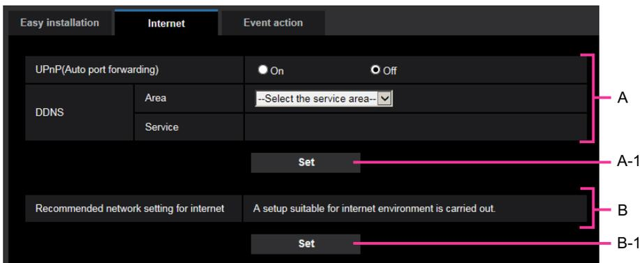
When completing the setting items in field ①, click the [Set] button ② below field ①). The edited settings in field ① will not be applied unless the [Set] button ② below field ①) is clicked. In the same manner as above, click the [Set] button ④ below field ③ when completing the setting items in field ③).
