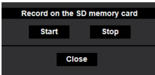
3. Click the [Start] button to start recording images on the SD memory card. The SD recording status indicator will light red (→page 12) while images are being recorded on the SD memory card. The image saving interval can be configured on the [SD memory card] tab of the “Basic” page. (→page 62)
