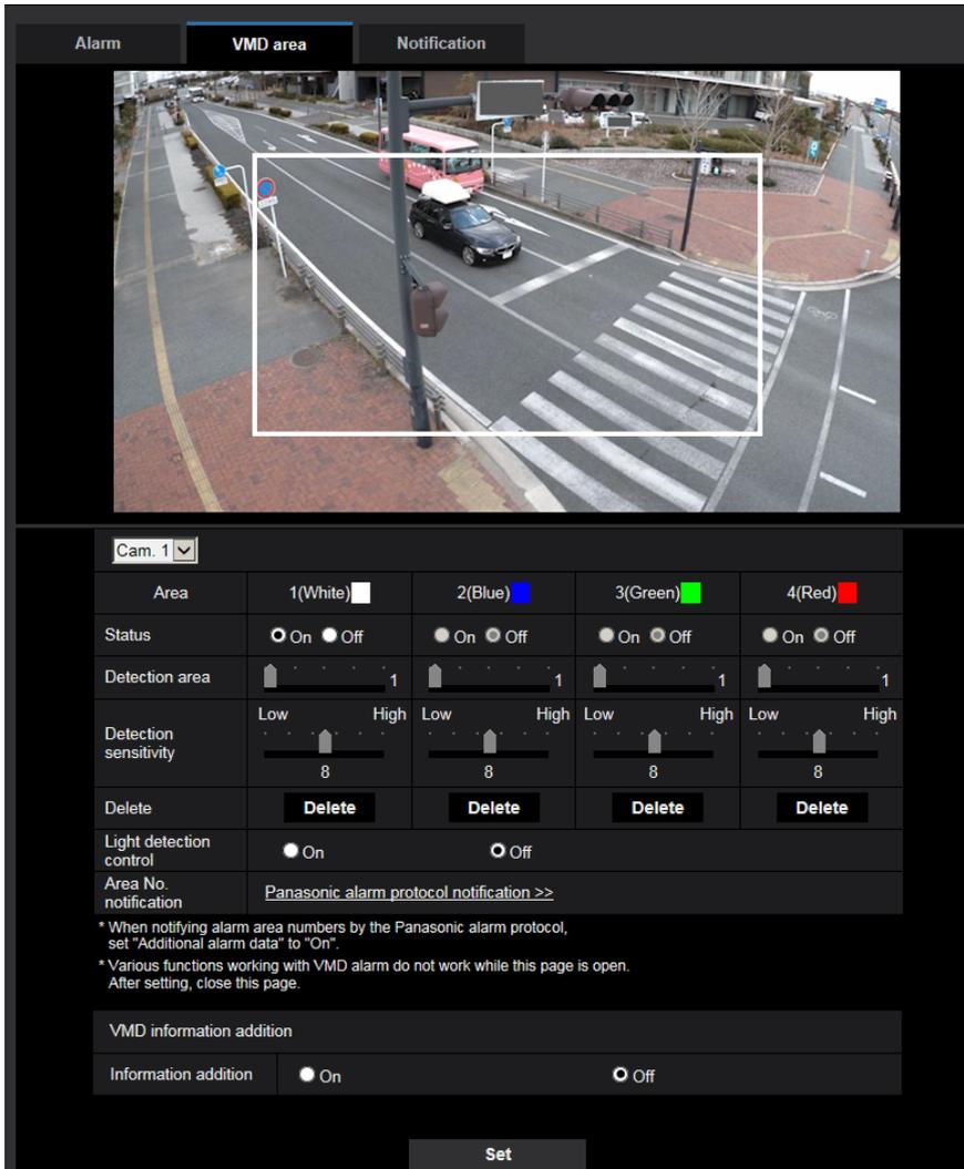
2. Adjust “Detection area” and “Detection sensitivity” using the slider.
