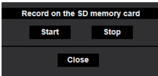
3. Click the [Start] button to start recording images on the SD memory card. The SD recording status indicator will light red (→page 13) while images are being recorded on the SD memory card. The image saving interval can be configured on the [SD memory card] tab of the “Basic” page. (→page 72)
