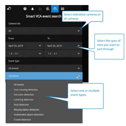
4. Click the Search button to begin the search. Depending on the scale of the search (how many cameras involved, and the span of recordings in search), the search should be completed in a few minutes.
