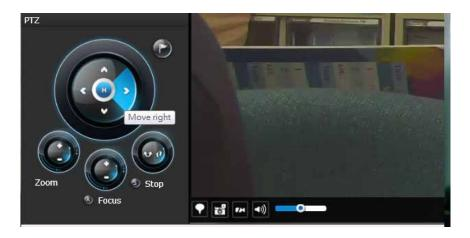
The preset positions and the patrol functions require the associated configuration on the cameras via a web console. Before you make use of these functions, you should set up the preset positions on a web console with the camera. The NVR GUI does not provide the configuration options with PTZ preset positions.
