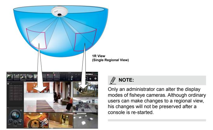
In addition to fisheye cameras, if a camera has a wide field of view, you may also display its different fields of view in multiple view cells. Some view cells may also contain a PiP view that is digitally zoomed.
