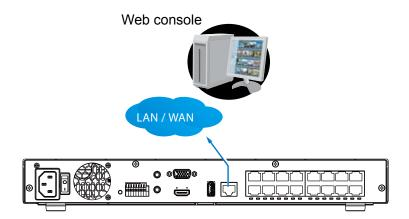
Note that when accessed over the network, the total streaming throughput is 96Mbps.
