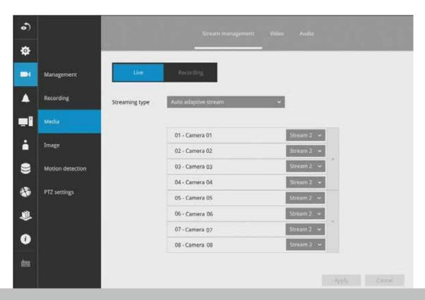
The NVR adaptively selects to display a video stream of a different resolution when it is displaying on a smaller view cell or a full screen.
