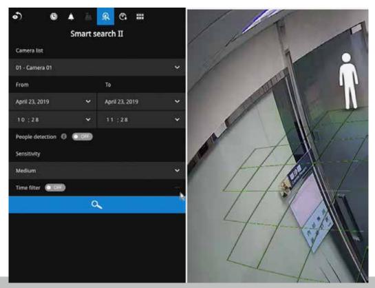
Click the Search button to begin the search. Depending on the scale of the search (how many cameras involved, and the span of recordings in search), the search should be completed in a few minutes.
