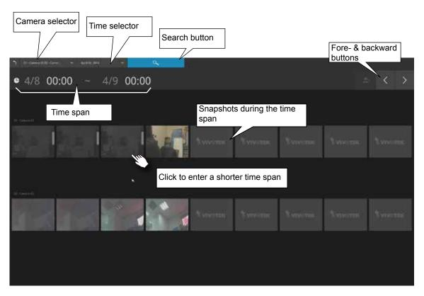
To search for a particular video footage, select the target cameras and the time of recording. On the Storyboard, the timelines of up to two cameras can be displayed.
