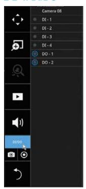
The DI/DO panel provides a glimpse of all DI and DO signal statuses from the connected cameras. You can manually trigger a digital output by clicking on its indicators.
