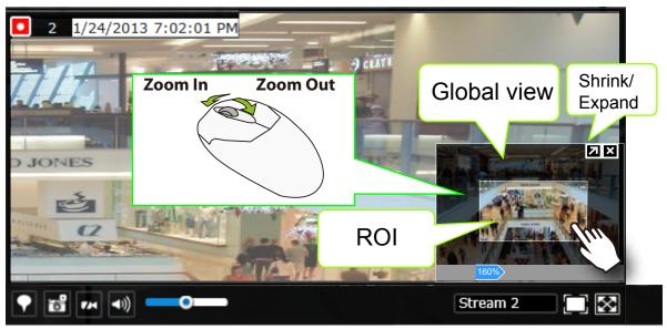
Note that not every camera supports the PiP function. For example, PTZ cameras do not support the PiP feature.
