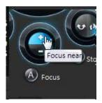
**Auto Focus**: If your camera supports the auto focus function, use this button to acquire an optimal focus point.
