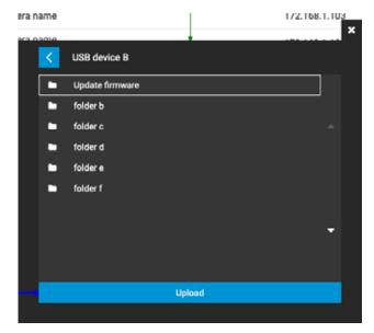
The Batch upload function allows you to update the firmware of multiple cameras. The firmware update can take place on up to 8 cameras at a time. The Waiting... message will display for cameras that are waiting for the update to take place.
