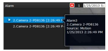
The alarm playback window will begin playback of a footage taken **10 seconds** before the occurrence of an alarm. The playback of an alarm-triggered recording will normally last for **one minute**. If, however, you configured a shorter pre- and post-alarm recording time, your alarm recording may be slightly shorter. The default for **pre-** and **post-alarm** buffer time are 5 seconds and 20 seconds.
