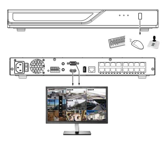
By default, a live view appears on an HDMI monitor. The interface architecture of the local console is illustrated as follows:
