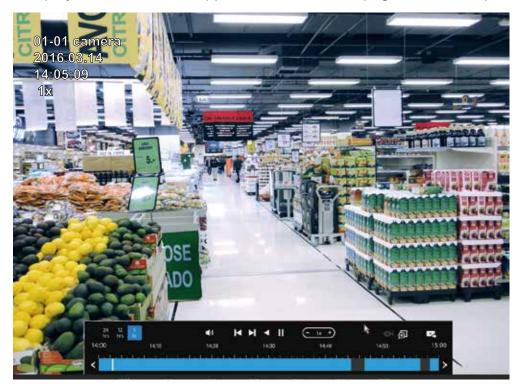
To return to the Live View window, click on the Back to Search recording clips button and the Back to Liveview button on the upper-left of the screen.
