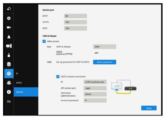
Instead of a web console, you can also access the NVR and the subordinate cameras using the **iViewer** and VIVOTEK's **VAST** software. The NVR can be managed as one of the sub-stations in a hierarchical device structure.
