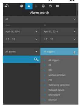
When done with the selection, click on the Search button. In the sample screen below, a list of alarms is displayed, and you can click on any of them to replay the moment when the alarm was triggered. The alarm-related recording will typically include a length of 5 seconds of pre-alarm and 20 seconds of post-alarm footage.
