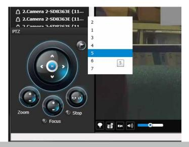
You can use **Preset** button to display preset positions and tell the camera to move and point at the preset direction, and to perform a camera tour to visit these positions in a consecutive order.
