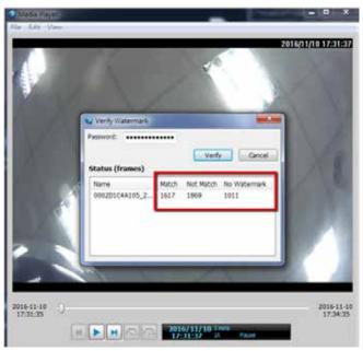
Enter the password to verify. If the Not match value is 0, the video is the original and has not been tampered with.
