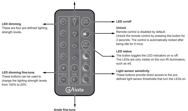
After a preset beam angle is selected, use these buttons to fine-tune. T stands for tele, W for wide.
