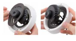
Now take the disc and pull it gently apart at the cut. Place the disc around the cables where the sealing and the housing meet. Push the disc down on the opening in the housing.
