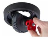
After initial operation of the camera, remember to adjust the focus of the lens (see «Initial Operation» on page 2).
