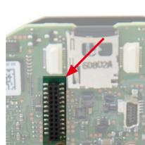
Use one finger to carefully press the board of the module onto the receptacle. Make sure that the Mx-A-IOA-IC is fully inserted.
