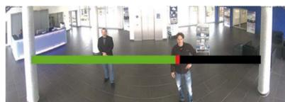
Carefully turn the lens using the red lens wrench in clockwise or counter-clockwise direction until the red area of the focusing aid in the camera image is as small as possible.
