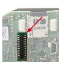
Use one finger to carefully press the board of the module onto the receptacle. Make sure that the Mx-A-IOA-IC is fully inserted.
