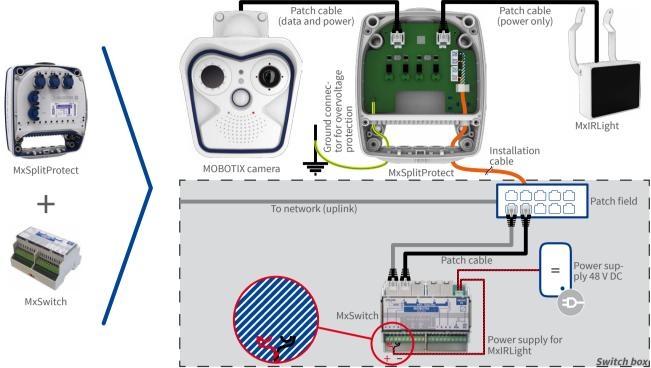
2. Split function for attaching two MOBOTIX cameras via an eight-wire installation cable for outdoor applications
