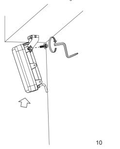
You will need to turn on both the partner camera and illuminator to precisely match the illuminated area with the camera's field of view. If necessary, adjust the beam angle again.
