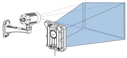
Turn the illuminator toward the FOV of the partner camera, shift the tilt angle, and then tighten the screw and the rear cover to secure the illuminator.
