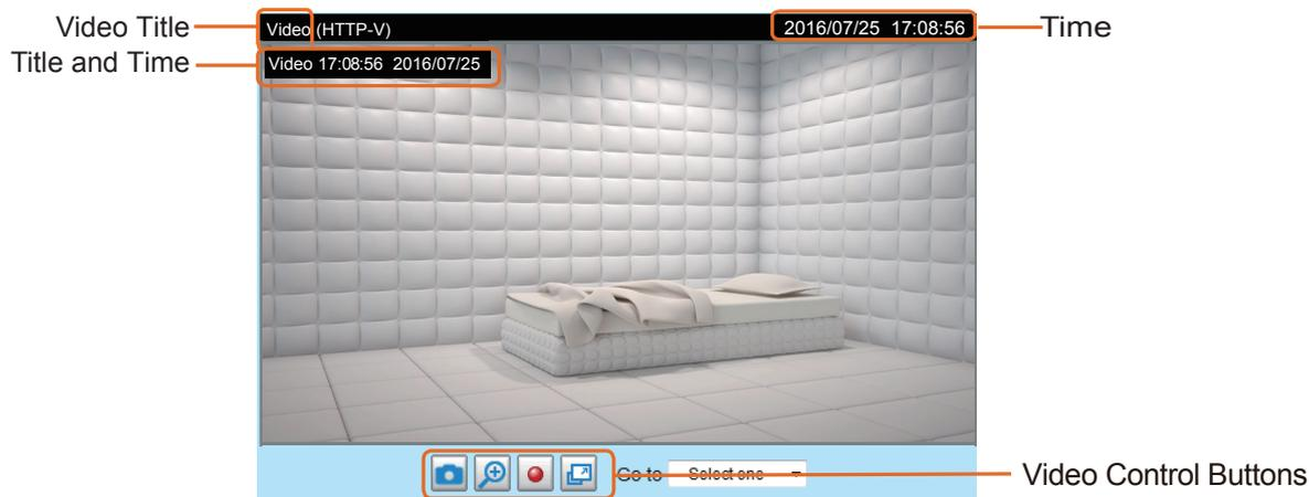
**Video Control Buttons:** Depending on the Network Camera model and Network Camera configuration, some buttons may not be available.
