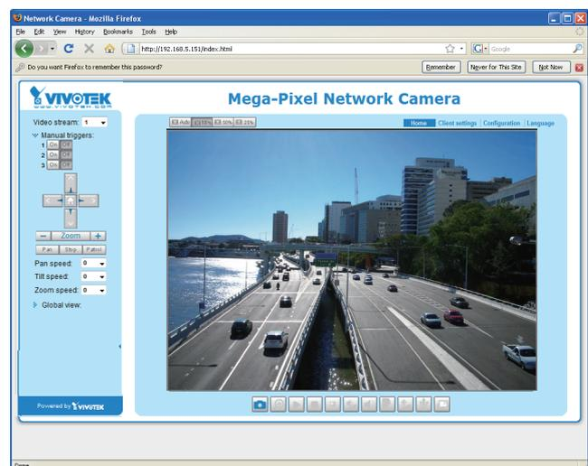
► *By default, the Network Camera is not password-protected. To prevent unauthorized access, it is highly recommended to set a password for the Network Camera. For more information about how to enable password protection, please refer to Security on page 90.*
