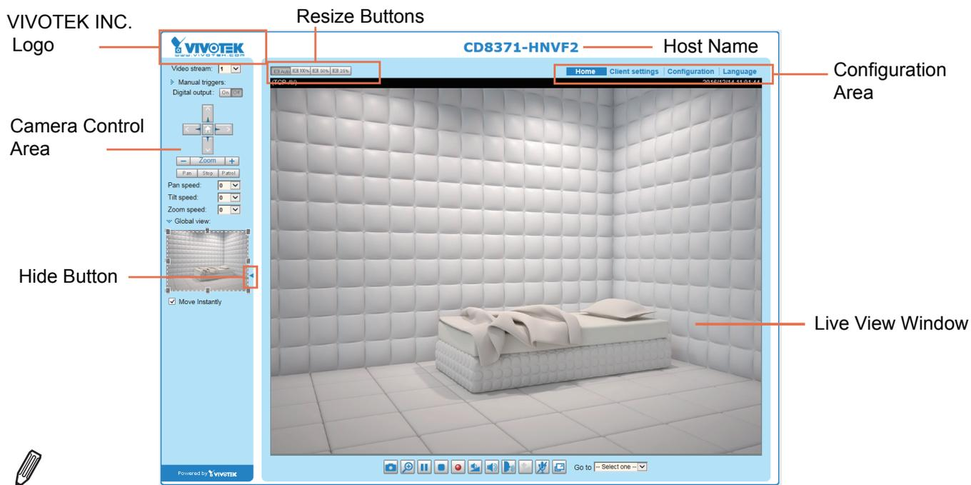
The Camera Control Area, the ePTZ control, is only available for stream #3.
