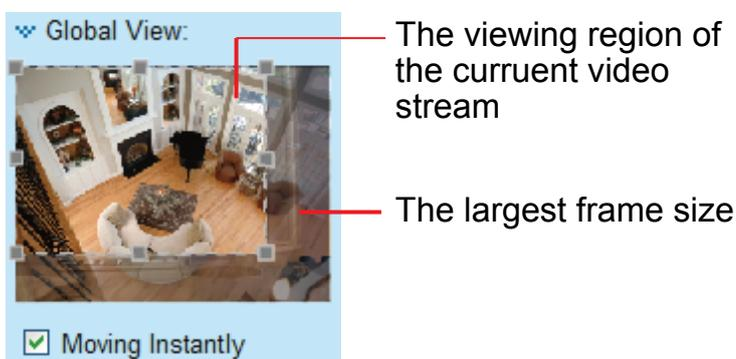
Note that the PTZ buttons on the panel are not operational unless you are showing only a portion of the full image. If the live view window is displaying the full view, the PTZ buttons are not functional.
