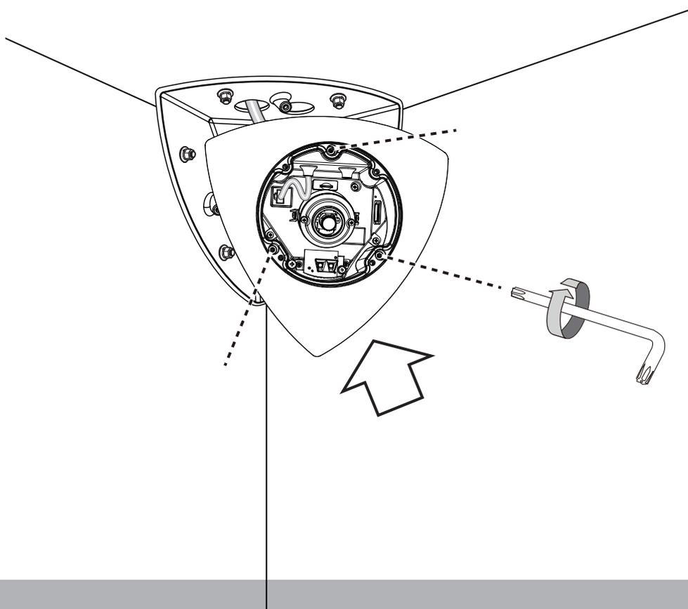
11. Insert a MicroSD card. Replace the desiccant bag with the one that comes with the shipping package.
