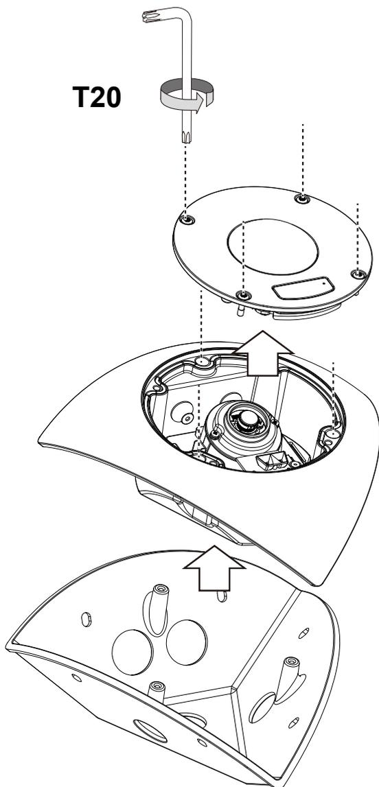
3. Use the base bracket as a template, and draw drill holes using a pencil. The camera is designed to be installed to a 3-sided corner of a room.
