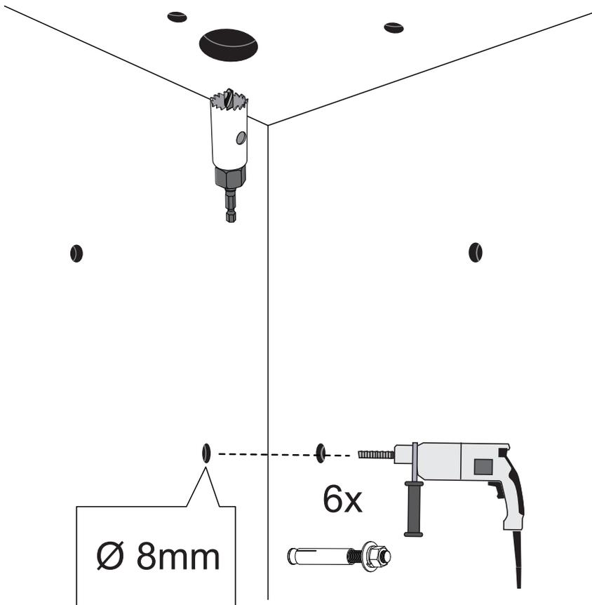
5. With threaded anchors in walls, secure the bracket to walls using hex nuts and washers.
