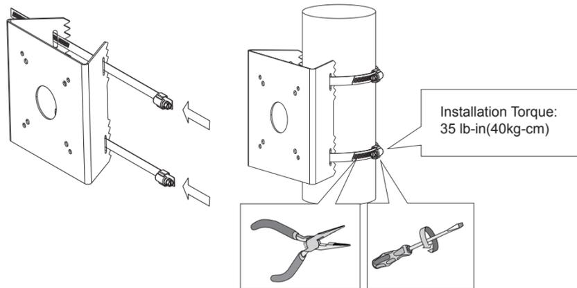
3. The 4 screw holes in the center are used for directly mounting the IB series bullet cameras.
