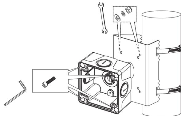
If you are installing a bullet camera directly to the bracket, use the M6 screws in the center. A hex crescent wrench is required.
