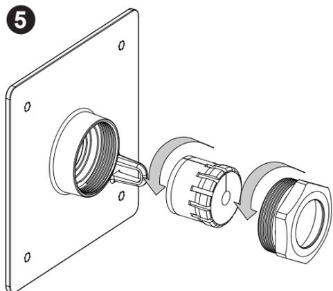
Install the rubber seal, claw, and sealing nut to the combo cable. Tighten up the sealing nut as shown below.
