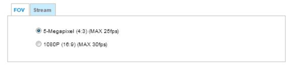
Select a resolution from the list. The default is 5 Megapixels, and if bandwidth or frame rate per second is of the concern you can select a lower resolution. You can configure the FOV to 1080P (16:9) at 30fps.
