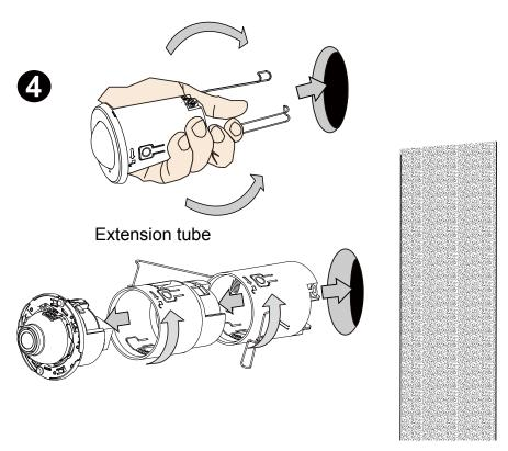
Use an extension tube if the wall is thicker than 6cm.
