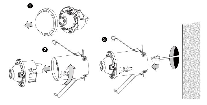
Pull the retention clips to the back of the module, and then insert the module into the wall.
