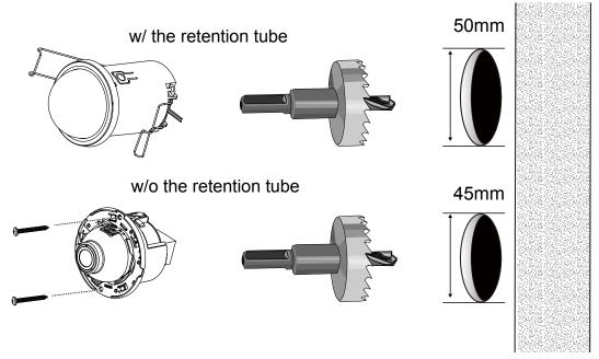
Use the M3 self tapping screws if installed without the retention tube. Note that this type of installation does not apply to hard surfaces, such as a concrete wall.
